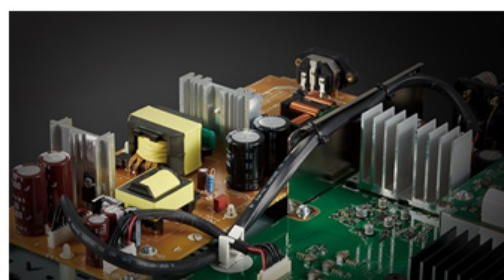
Twin Power Supply Circuit
