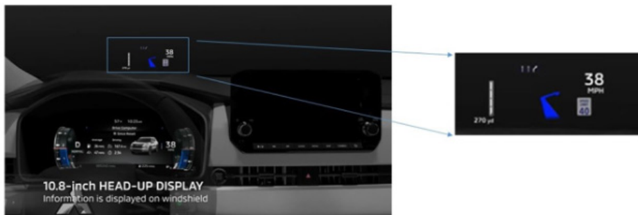
HUD screen image projected onto a windshield (Photo courtesy of Mitsubishi Motors Corporation)
