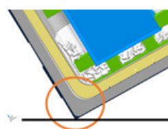
Buffer layer absorbs shock when dropped
