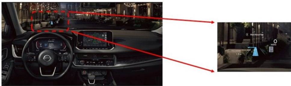
HUD screen image projected onto a windshield (Photo courtesy of Nissan Motor Corporation)
