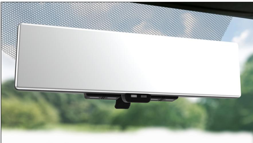
4. Camera is positioned at the rear window. No projection of back passengers reduces blind spots and improves rearward visibility.
