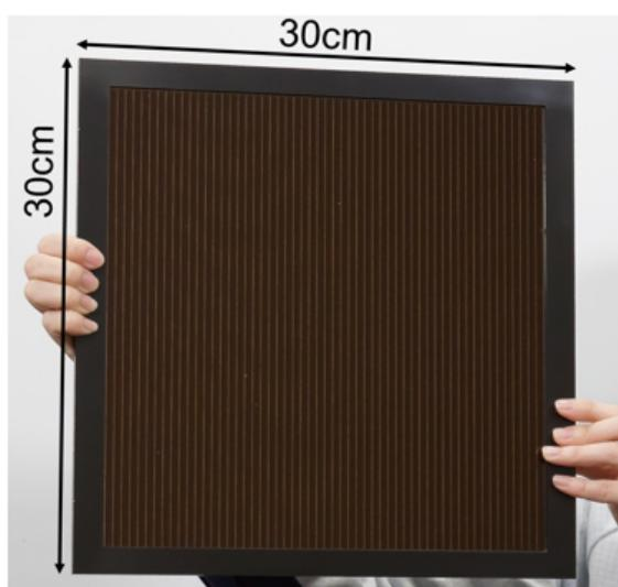
Fig.1 Perovskite module with the world's highest conversion efficiency among that of the same size
