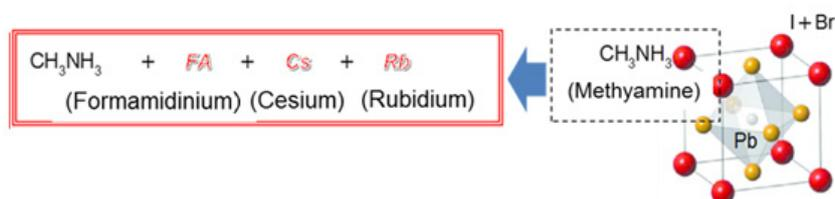
Fig.2 Perovskite crystal
