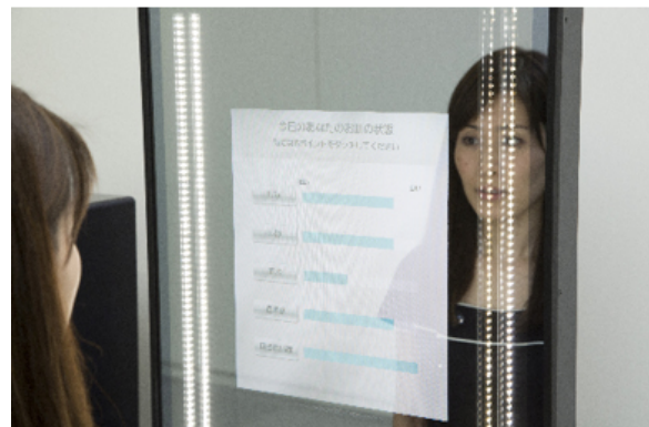
Snow Beauty Mirror (Displays the results of skin analysis covering five categories)
