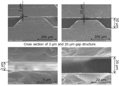
Detailed view of gap structure of 3µm and 20µm
