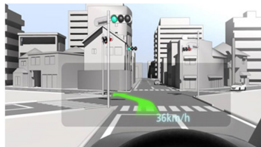
The guidance display of car navigation is superimposed on the actual scenery and displayed more clearly. Reduce driver's viewpoint movement and reduce physical burden.
