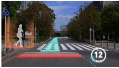
The HUD system detects and highlights pedestrians to attract the driver's attention.
