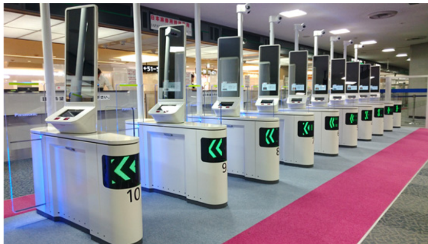
Panasonic automated facial recognition gates at immigration examination area in Narita Airport Terminal 1 Building (South Wing)
