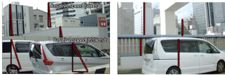
Rolling shutter Global shutter Fig.7 Comparison of shutter modes Highway driving
