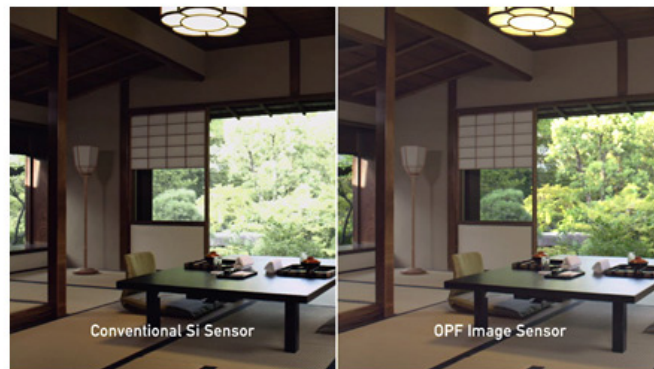
Conventional Si image sensor OPF image sensor Fig6. 8K sensor Wide dynamic range imaging Japanese room
