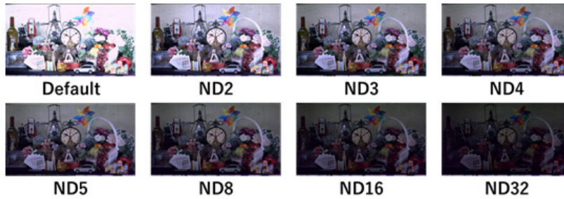
Fig. 11 Electrical ND Filter Imaging Studio
