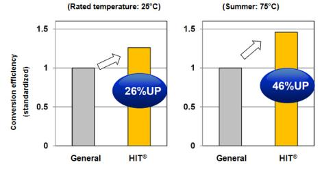
\* Calculated based on a conversion efficiency of 15.6% and output temperature coefficient of -0.50%/°C for general silicon solar cells and a conversion efficiency of 19.6% and output temperature coefficient of -0.258%/°C for HIT®.
